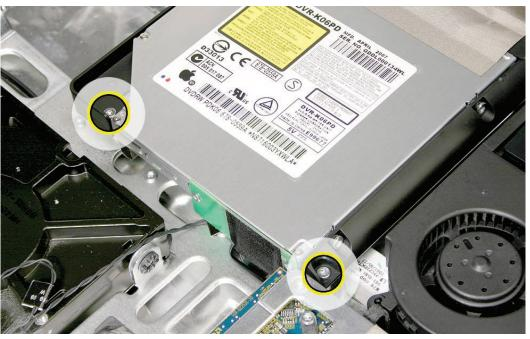
2. Carefully peel back the strip of EMI mesh tape that anchors the bezel end of the drive to the
